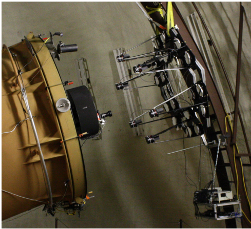
Fig. 1. SCALA attached at the ladder of the dome of the UH88 telescope. The projector modules with the three mirrors and the IS hold in front of them are visible in the image, below SCALA is located the lamp+monochromator system and the electronics boxes.
